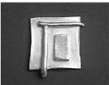
**Overlays & Joints** In many cases, connections can be made by overlapping pieces of PMC. Often the pieces are simply layered into position and lightly pressed together. If the clay is starting to dry, add a tiny drop of water with a brush at the edge of the overlay. When a situation offers less contact, dampen the two surfaces to be connected with a drop of water and texture them with fine lines
